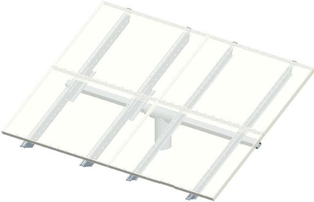
**5:** Lift the Assembled Solar Mounting and fit the Cross pipe section into your 4" pole adjust the whole unit to face the optimum direction of sun light. Tighten down the Single M16 Nut to prevent the unit from swirling. Then adjust the Angle of the Guide rail to the appropriate degree of incline based on the location of your installation to optimized sun light condition. Tighten down the 2 x M16 Hex bolts after the optimum angle has been reached as shown in the Diagram.
